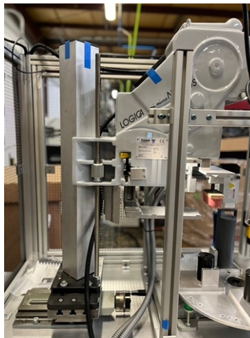
Mounting post with Z axis adjustment on top of the TO-200 XY cross table.
