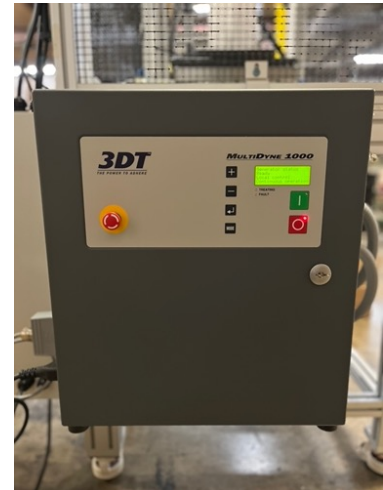
3-DT corona pre-treatment electrical / generator.
