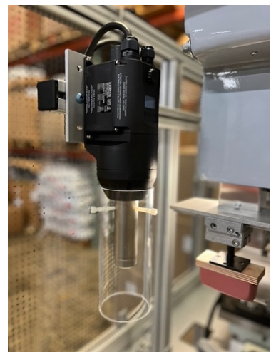
Leister hot air gun head mounted using 80/20 for X and Z axis adjustment over part on rotary dial.
