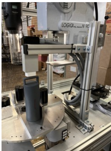
3-DT corona pretreatment head mounted using 80/20 for X and Z axis adjustment over part on rotary dial.
